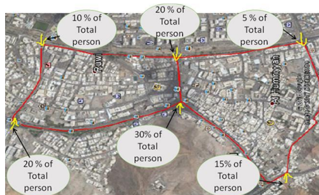
Fig. 6: Geographical distribution of traffic entry at the Gateway points to City Center
