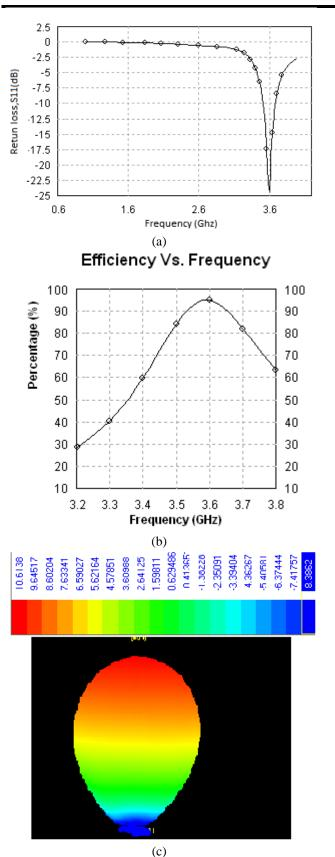
Fig3 (a) Return loss result at 3.6Ghz resonating freq.(b)Efficency versus Frequency.(c) 3D Radiation Pattern of standard microstrip rectangular patch antenna
