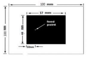
Fig.2: Geometry of top view the high gain Rectangular Microstrip patch Antenna
