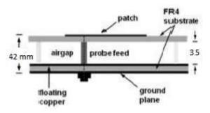
Fig.1: side view of double layer with air gap
