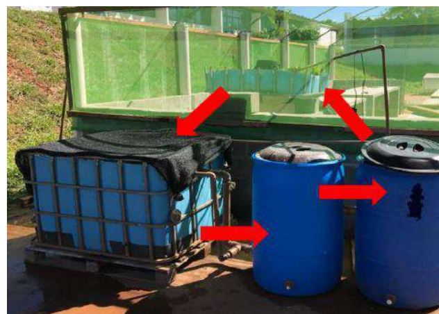
Fig. 5: Intensive recirculation system.
