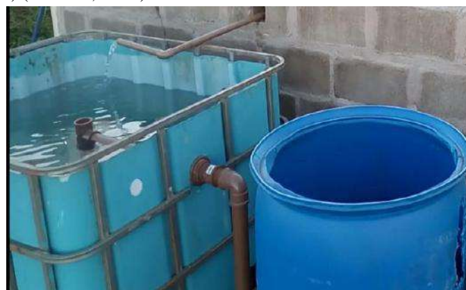
Fig. 2: Model of IBC container used in the aquaponics pilot system.
