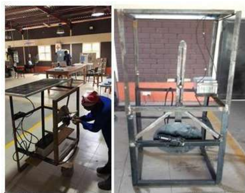
Plate 8: Solar-powered slider crank mechanism assembly before field test
