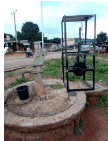
Plate 9: Solar-powered slider crank mechanism assembly during field test
