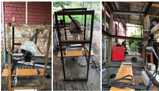
Plate 7: Different views of the fabricated solar-powered slider crank hand pump system
