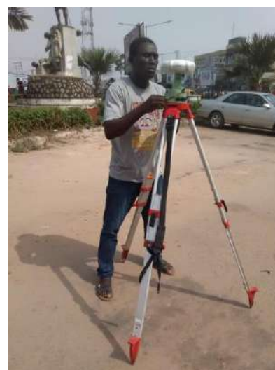
Fig. 6: Rover Receiver at One of the Selected Points (RR01) at Ring Road
