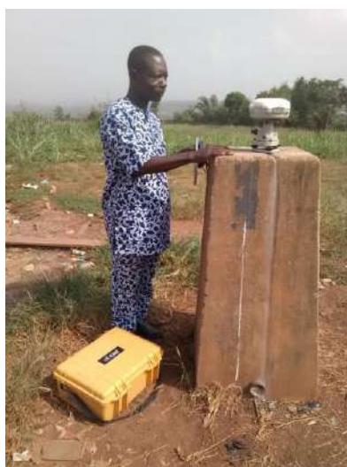
Fig. 5: Base Receiver at Control Station XSU92
