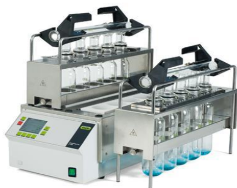
Fig.1: The Kjeldahl apparatus Buchi digester K 436/ K 439, in which the nitrogen is determined by the amino acid stain (Operation manual SpeedDigester K-425 / K-436)
