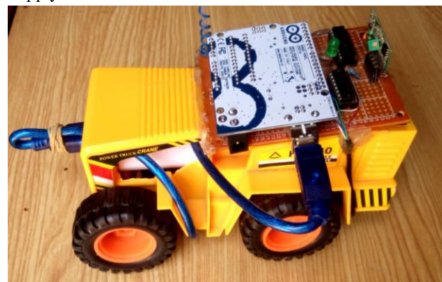
Fig.8: Robotic Car and Receiver Part Circuit
