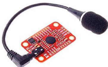
Fig.3: Microphone and voice recognition module
