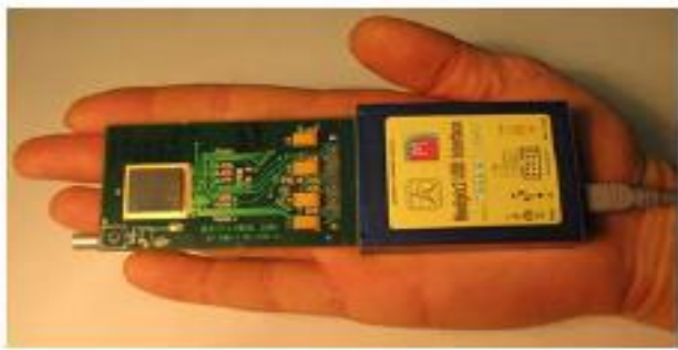
Fig.2: Compact portable set up with USB interface.
