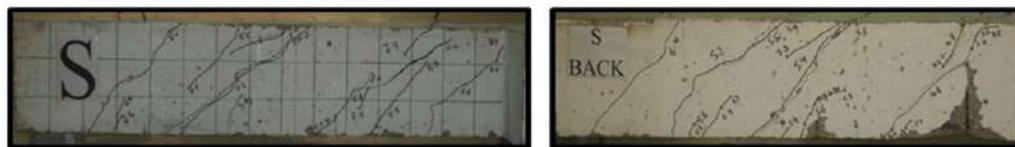
a) Crack pattern for the solid specimen
