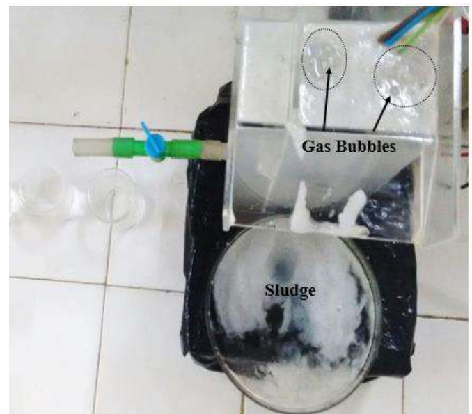
Fig.13: Top view of the electro flocculation reactor used in the treatment of wastewater for the purification of biodiesel after an experiment. (Source: research' image).
