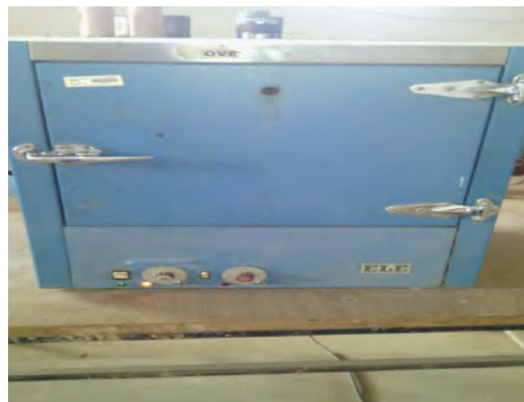
Plate III: Oven used for curing of the produced electrodes at Civil Engineering Lab. (FUT, Minna)
