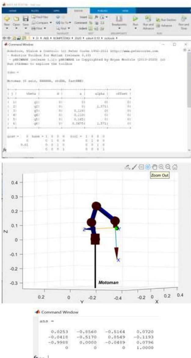
Fig. 6: Result of Forward Kinematics in Matlab
