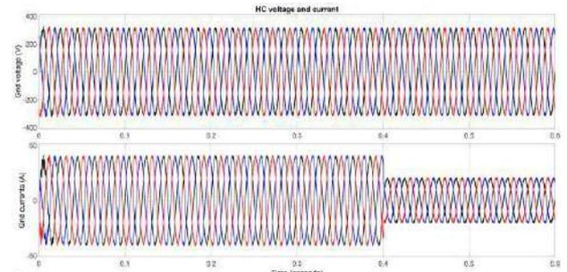
Fig. 13: Voltage and current response of the HC
