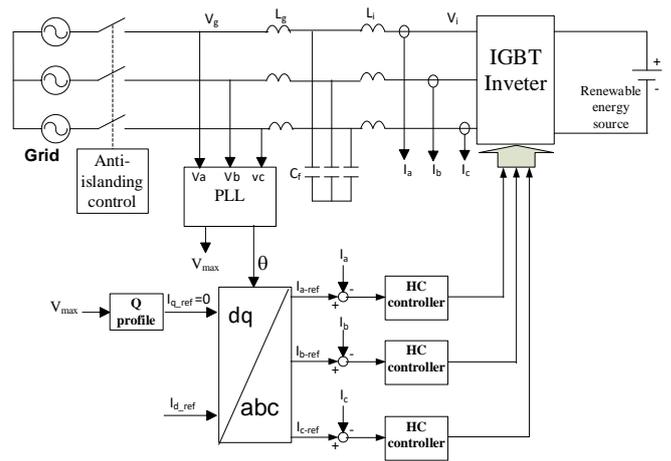
Fig. 1: Three-phase grid-connected inverter system using the HC controller.
