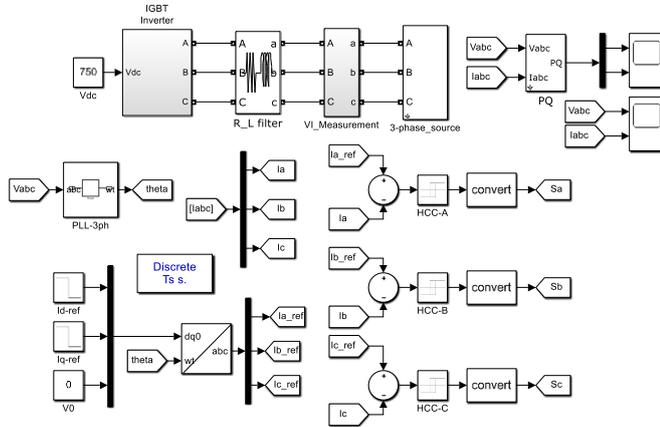
Fig. 4: Simulink model using the HC controller
