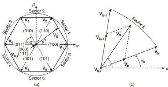
Fig. 8: The states and principle of space vector
