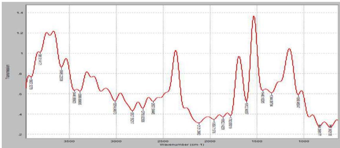
Fig. 6: FTIR Spectrum of the formulated self healing paint
