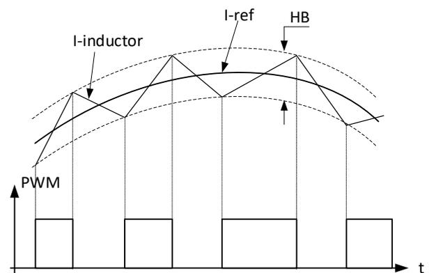
Fig. 3: The switching principle of the HC controller
