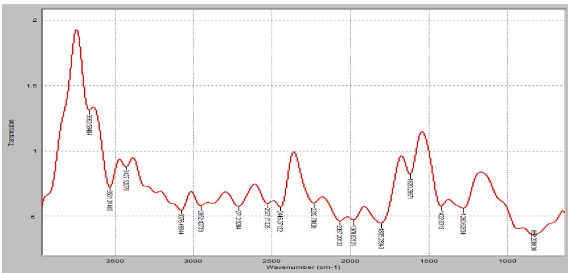
Fig. 4: FTIR Spectrum of Chitosan-g-maleic anhydride-g-(Methyl methacrylate)
