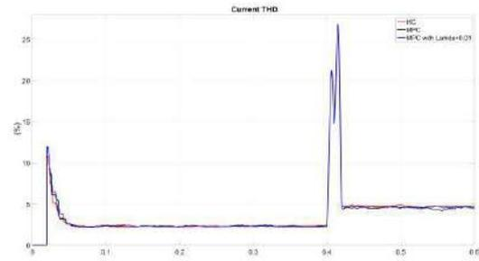
Fig. 17: Current THD of HC and MPC
