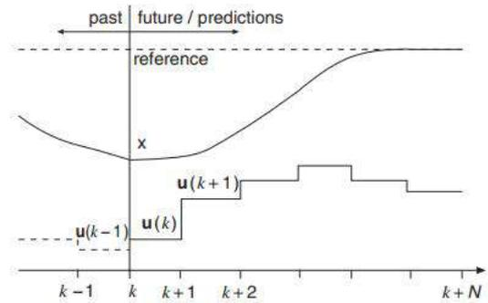
Fig. 7: The operational principle of MPC
