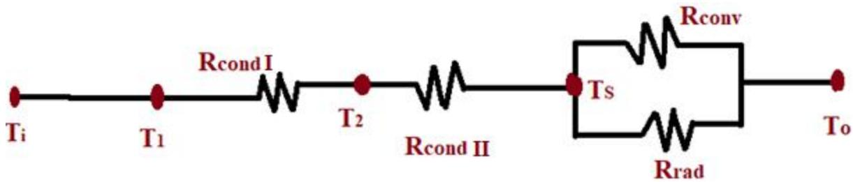
Fig.6: Kiln shell resistance equivalent circuit diagram
