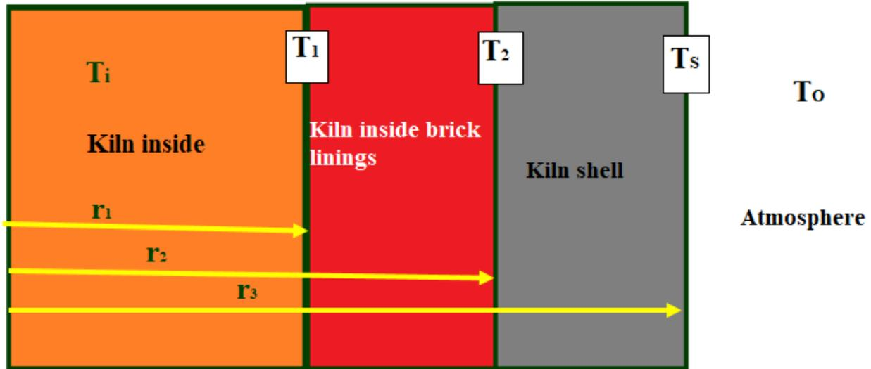
Fig.5: The rotary kiln shell longitudinal cross section
