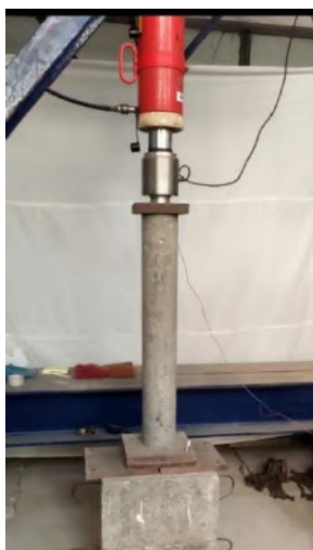
Fig. 4. Setup testing of the pile specimens.
