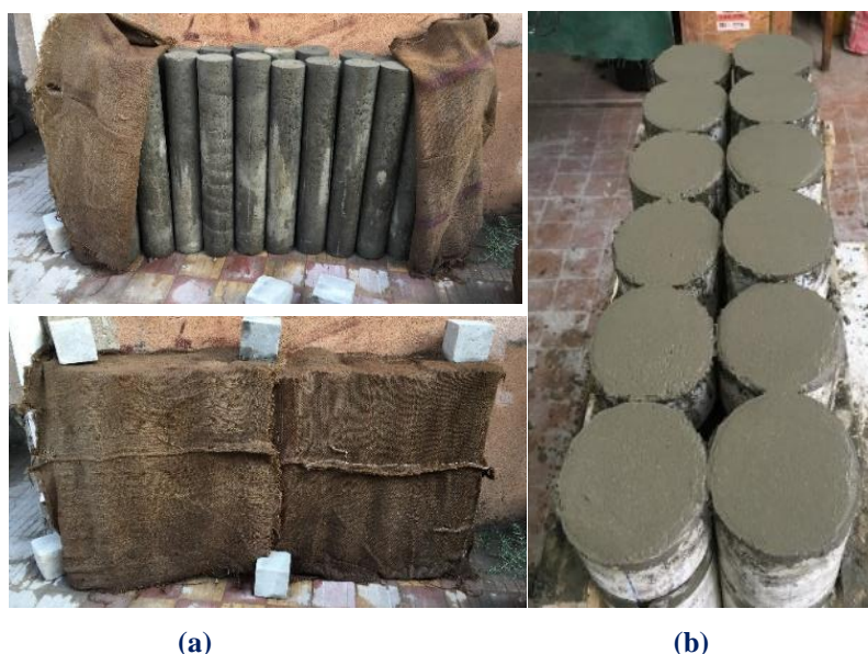
Fig.2: (a) curing conditions, (b) pile models.
