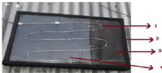
Fig.2 : Components of a flat-plate glazed collector.
