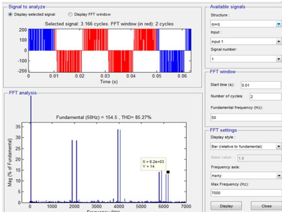
Fig.8: Fourier analysis of inverter output
