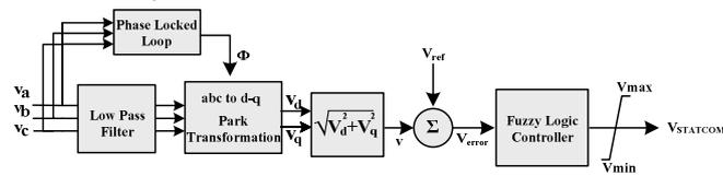
Fig.4: Block diagram for STATCOM control system
