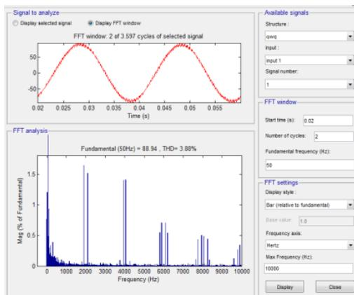
Fig.9: Fourier analysis of line current after STATCOM voltage injected
