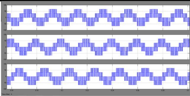
Fig.7: The 3-ph phase waveforms output of the inverter
