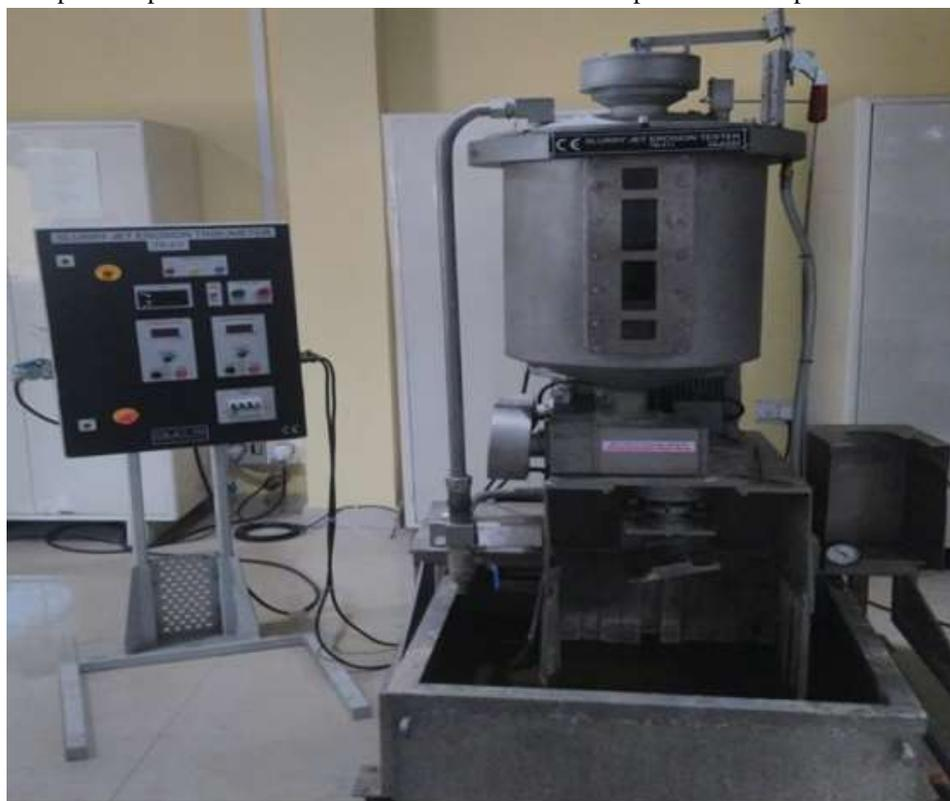
Fig.2: Test setup of Slurry Jet Erosion Tester
