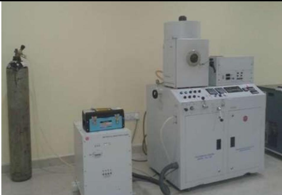
Fig.1: Thermal/E-beam PVD Coating Unit
