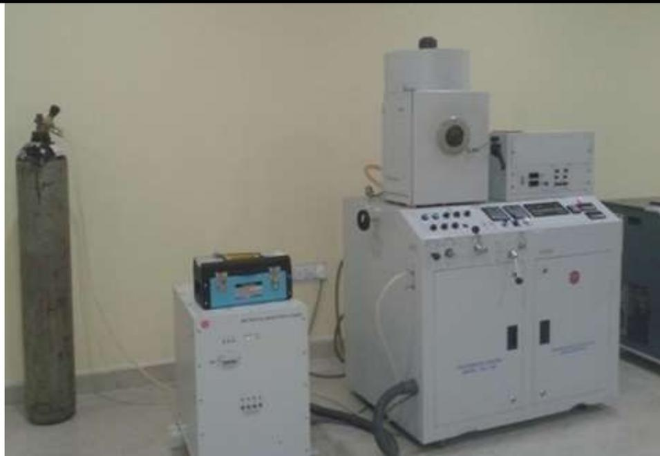
Fig.1: Thermal/E-beam PVD Coating Unit
