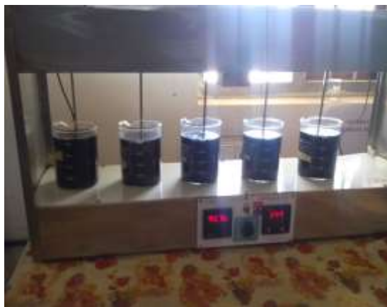
Fig.1 : Jar Test Apparatus with Leachate Samples
