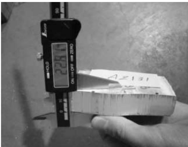
Fig.3: Cross section of roll casted AZ131 strip
