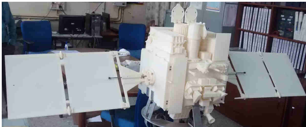
Fig.9: Completely assembled ASTROSAT model in deployed condition.
