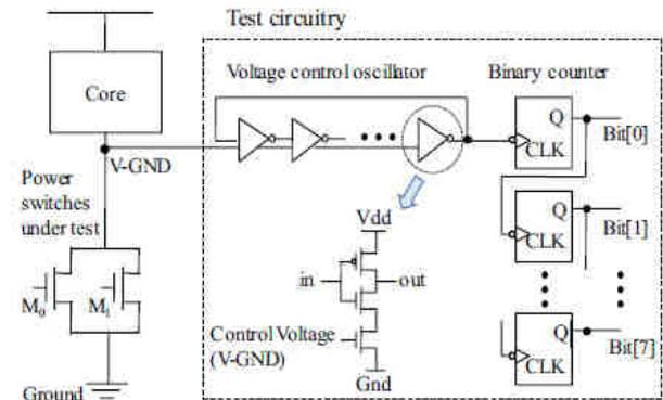
Fig. 4 Proposed Multimode Power Switch Circuit
