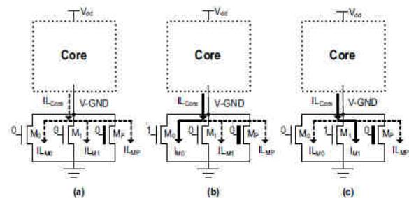
*Fig. 3 Multimode Power Switch Circuit*
