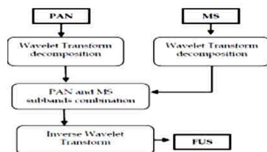
Fig. 5.1. Block diagram of the Wavelet fusion method.
