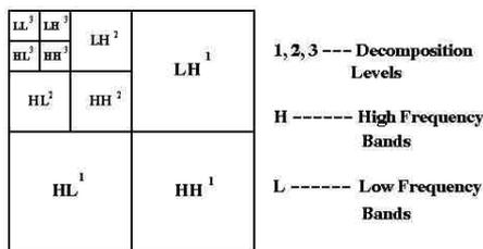
Fig. 5.2. Decomposition of DWT Levels
