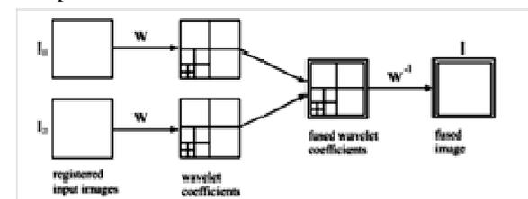
Fig. 2.1: DWT Image Fusion Process flow diagram.
