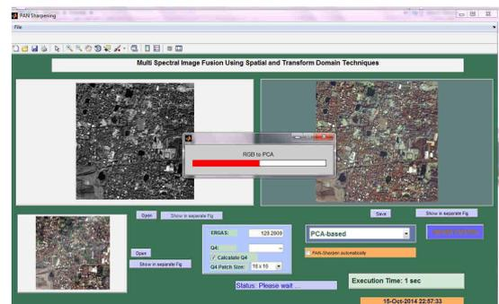
Figure 6.5: PCA based image fusion
