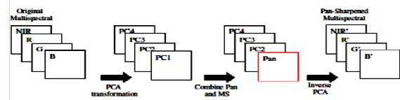
Fig. 5.4 PCA conversion of components
