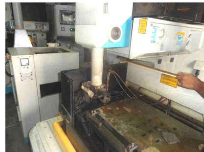
Figure 3.1 WEDM Setup for experimentation
