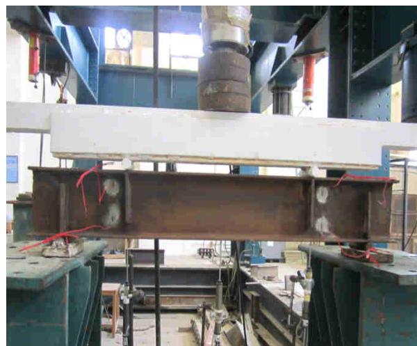
Fig. 4: Test setup for the control specimen (Bo).
