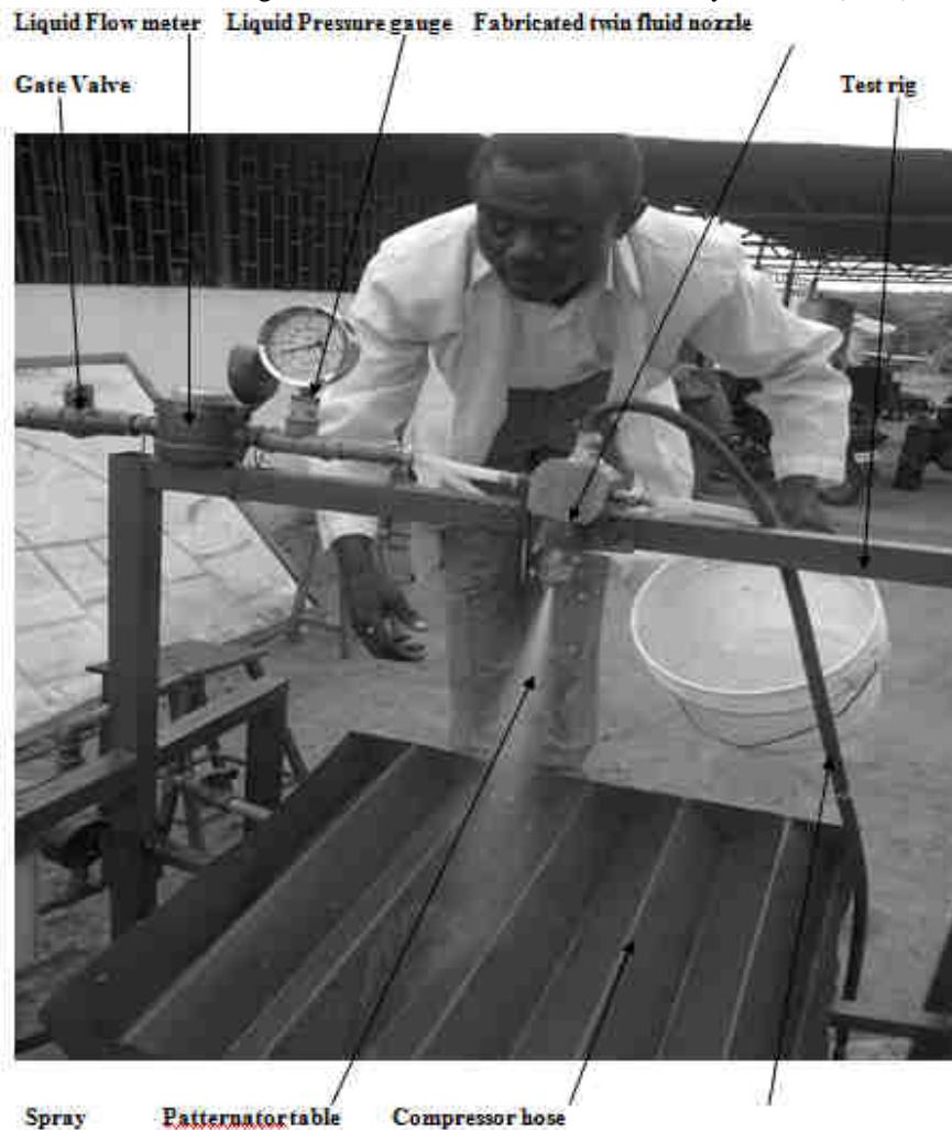
Fig. 6: Test setup for measuring the nozzle spray distribution pattern
