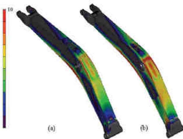
Fig.10: Isometric view of the boom models distribution over the upper plates (a) Initial model. (b) Optimized model
