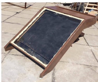
Fig. 3 The transparence solar air heater used in the study
