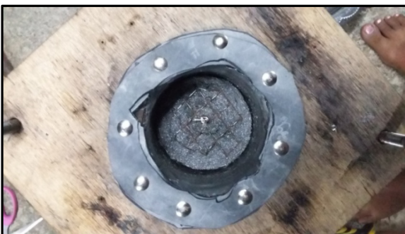
Fig 2: Setting piston inside the cylinder
