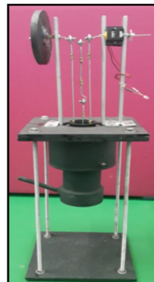
Fig 4: Flywheel with shaft attached to dynamo
