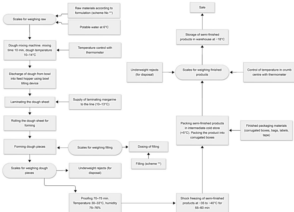
Fig. 1. Adapted technological scheme for the production of puff-yeast frozen semi-finished products
