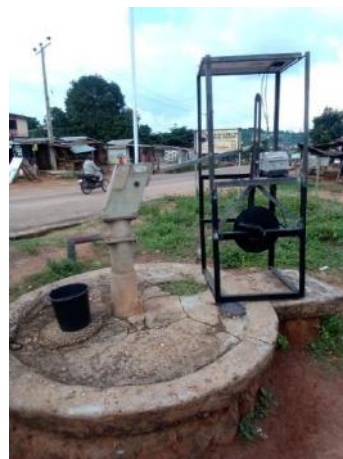
Plate 9: Solar-powered slider crank mechanism assembly during field test
