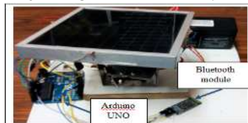
Fig. 5: Hardware Assembly with Bluetooth Module
