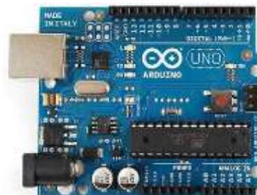
Fig. 2: Arduino Uno Microcontroller Development Board
