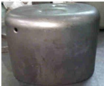
Fig 10: Hole Flanged Shell
