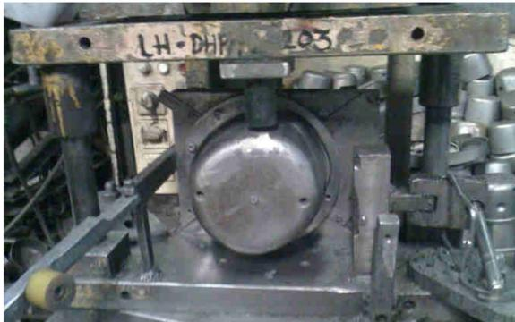
Fig 12: Hole Flanging Tool.
