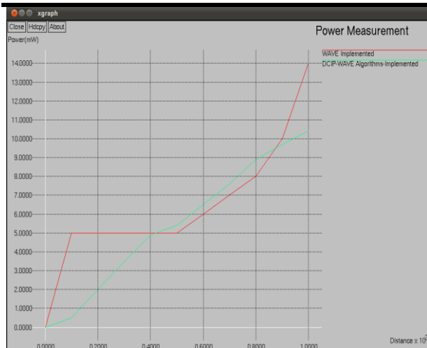
Fig.8. Decrease of Power consumption based on Distance between RSUs
