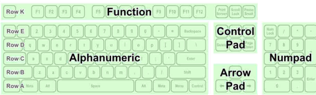
Fig. 1: The five general sections of a standard keyboard
