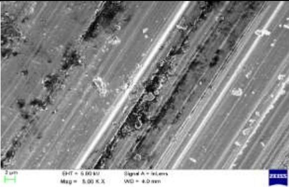
Fig.8: SEM Image for vacuum Tempering for 120 minutes
