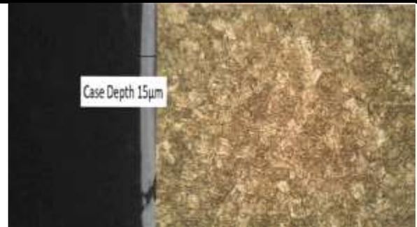
Fig.4: Vacuum tempering for 120 minutes 15 microns
