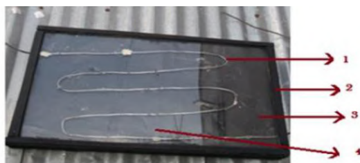
Fig.2 : Components of a flat-plate glazed collector.
