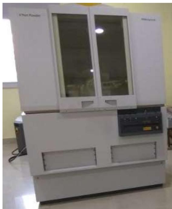
(a) Test setup of XRD machine
