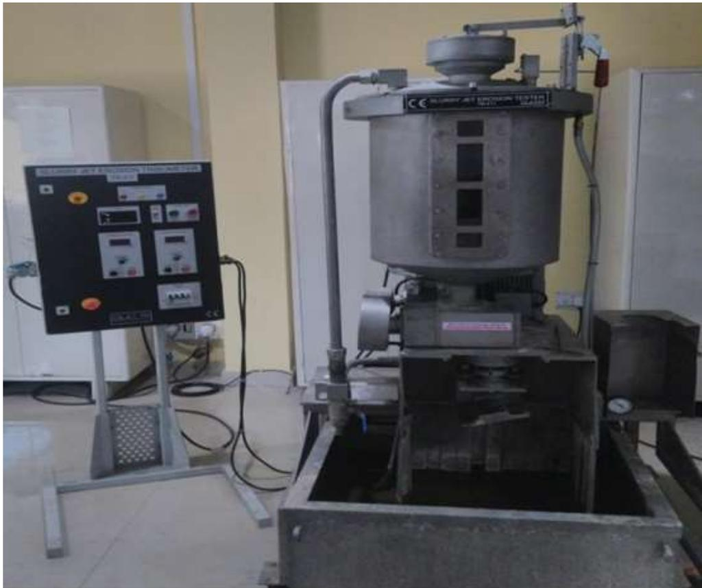
Fig.6: Test setup of Slurry Jet Erosion Tester
