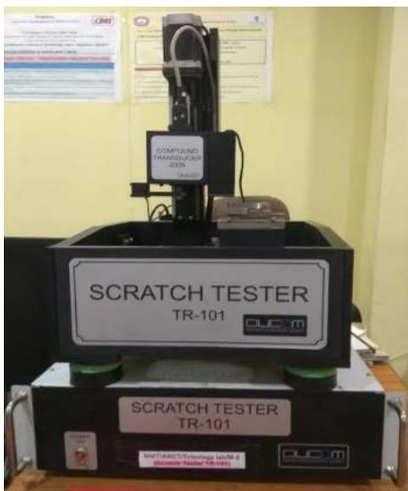
Fig.9: Test setup of Scratch Tester
