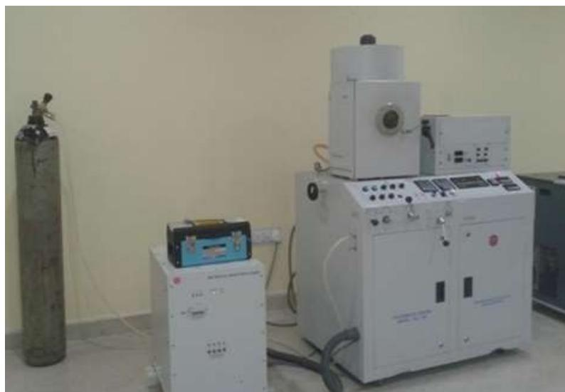
Fig.7: Thermal/E-beam PVD Coating Unit
