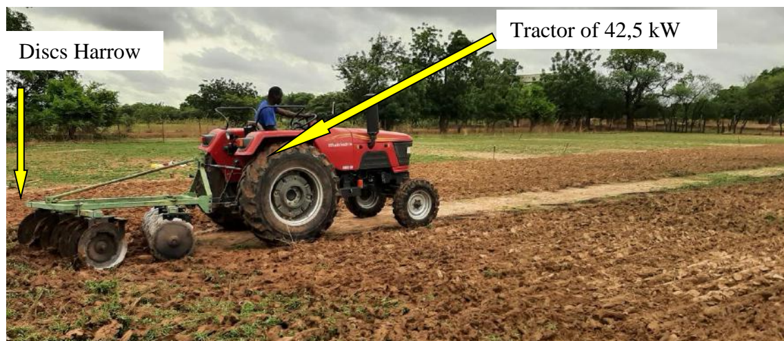
Fig. 1: Discs harrow hitched to the Mahindra 605 DI tractor during experiments.
