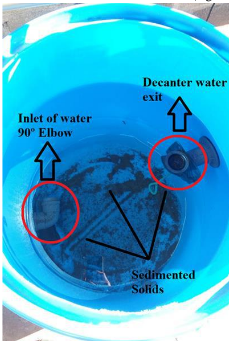
Fig. 4: Inlet and exit of the barrel with decanter function.
