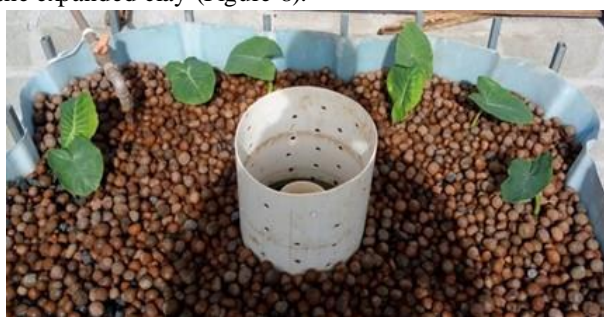
Fig. 8: Filter with stone gravel and expanded clay.
