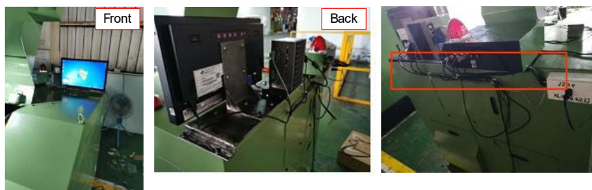
Fig10: Monitor Position (Front) & Computer Host and Monitor Mounting Bracket (Back) & Rear Cabling
