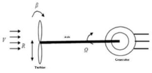
*Fig 3: Wind turbine model*
