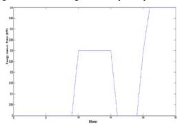
Fig 23: Daily functioning distribution of three generators according to load profile
