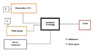
Fig 5: Hybrid system structure
