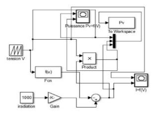
Fig 9: Block diagram of a photovoltaic cell.
