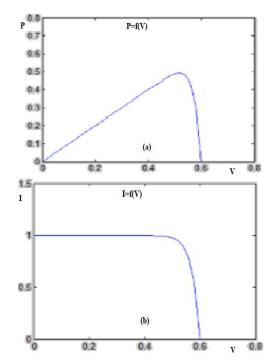
Fig 11: Characteristics of a cell for solar irradiation of 1000W/m2 at 25 ° C: (a) P = f(V), (b) I = f(V)
