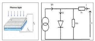
Fig 2: Photovoltaic cell equivalent circuit
