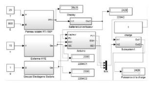
Fig 19: Block model of hybrid system on Matlab/Simulink
