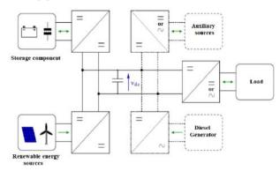
Fig 1: Hybrid system structure
