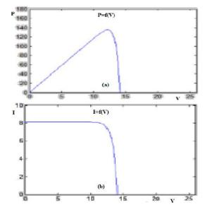
Figure 12: Module RT-150 p features: (a) power-voltage, (b) current-voltage
