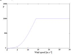
Fig 14: Wind turbine power variation over wind speed
