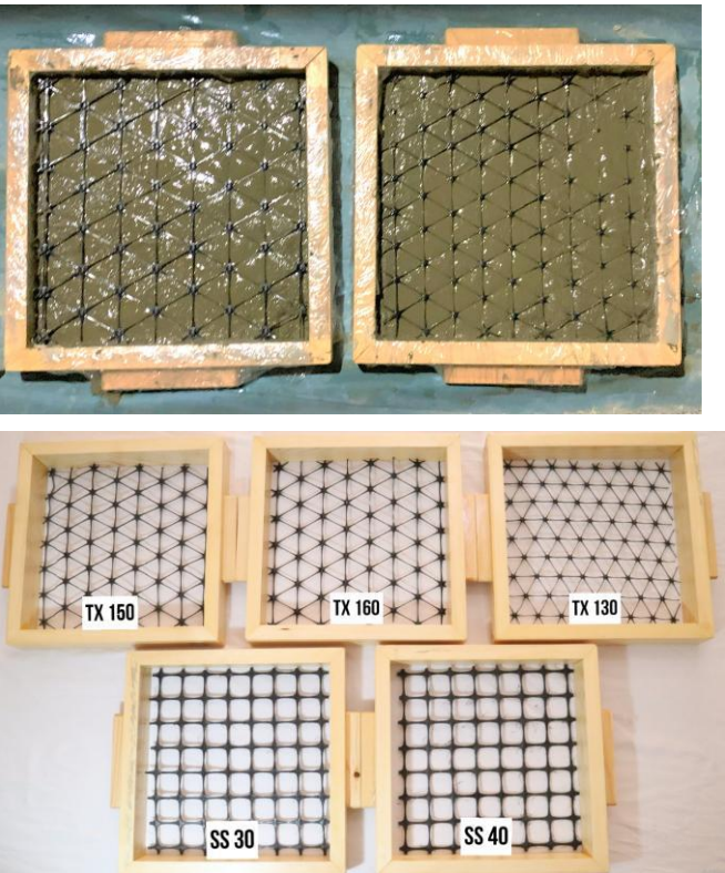
Fig.2. Placing of the geogrid layer after pouring and compacting of the 2.5 cm concrete layer,
