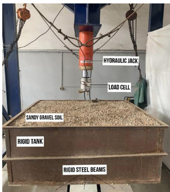
Fig. 3: Test Tank Configuration for Investigation of Footing-Soil Interaction.
