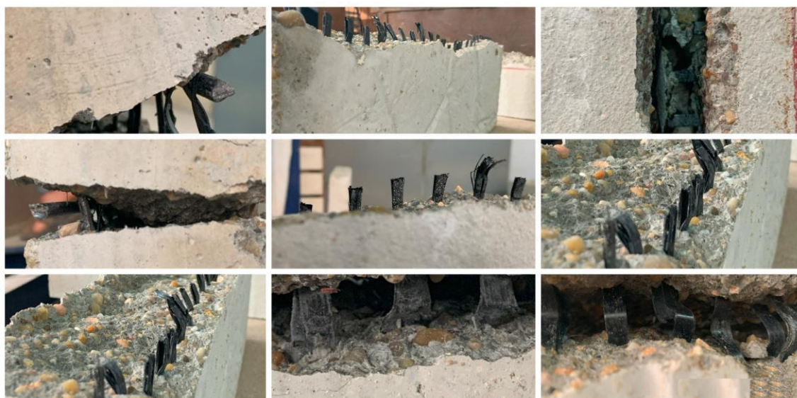
Fig. 14: Geogrids' Rib Status after Failure of Concrete Footings “showing the condition of geogrids' ribs following the failure of the footings”.
