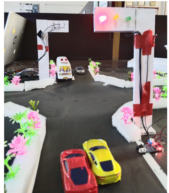
Fig. 6: Density based traffic light control system in operation
