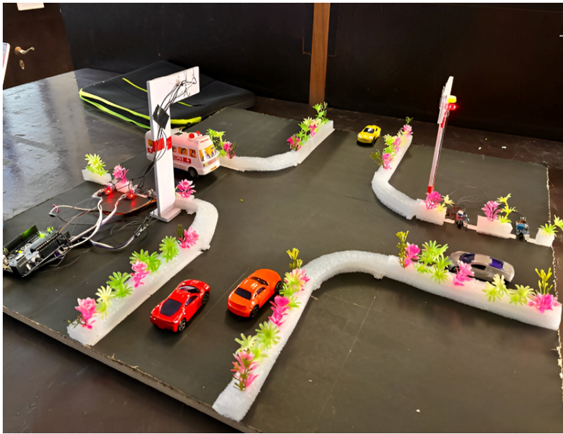
Fig. 6: Density based traffic light control system in operation
